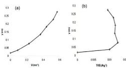
y = flow depth; U= downstream flow velocity; TKE = turbulent kinetic energy.
